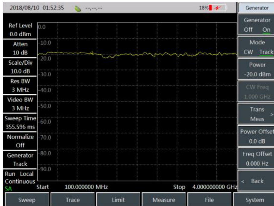
Fig. 4-26 Schematic diagram of tracking mode
