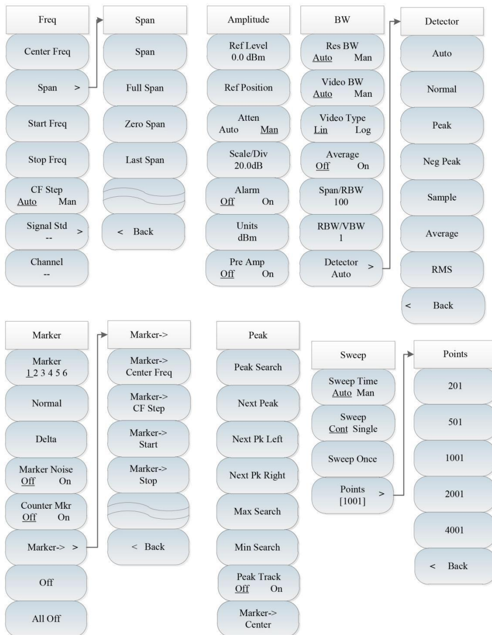
Fig.10-5 Block diagram of signal analysis menu
