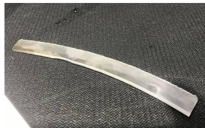
Arc-shaped silicon glass thick sample cutting (2mm thin slice)
