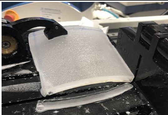
Arc-shaped silicon glass thick sample cutting (2mm thin slice)
