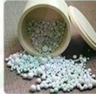
Corundum tank and alumina ball
