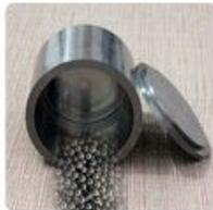
cemented carbide tank and balls
