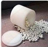
Nylon tank and zirconia balls
