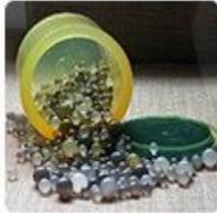
Polyurethane (pu) tank and agate balls
