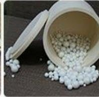
Corundum tank and zirconia balls
