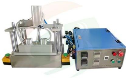
The battery pouch vacuum sealing machine TOB-JK-200 is mainly used for sealing aluminum-laminated case in glove box after injection of electrolyte into pouch Li-ion cell or after formation for final seal (polymer Li-Ion cell).
