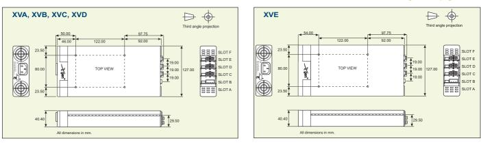
The XV family of medically approved power supplies provides up to an incredible 1340W in an extremely compact 1U package. Providing up to 12 isolated DC outputs, the XV family employs innovative plug & play architecture allowing users to instantly configure a custom power solution in less than 5 minutes!
