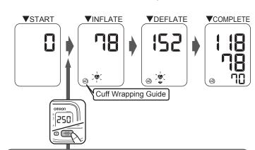
If your systolic pressure is more than 210 mmHg After the arm cuff starts to inflate, press and hold the START/STOP button until the monitor inflates 30 to 40 mmHg higher than your expected systolic pressure.
