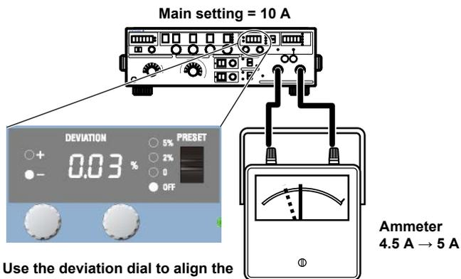
Use the deviation dial to align the meter needle to the accurate scale position.
