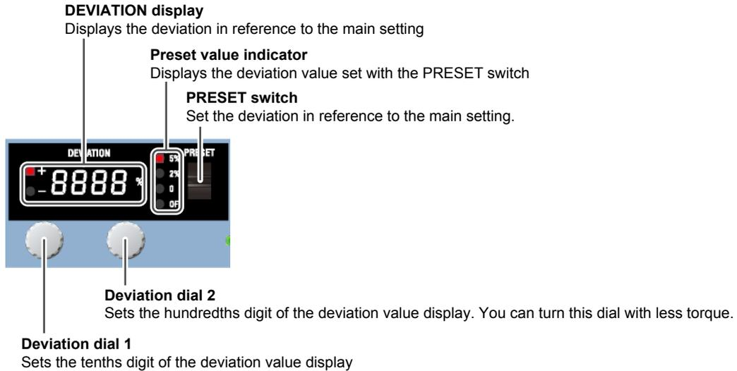
The deviation dial sets the number of each digit in the range of 0 to 9. Dial 1 changes the number in increments of 2; Dial 2 changes the number in increments of 1. Carrying over and borrowing occurs automatically up to  $\pm 20\%$ . If the upper or lower limit of the range is reached, turning the dial further will not change the number.
