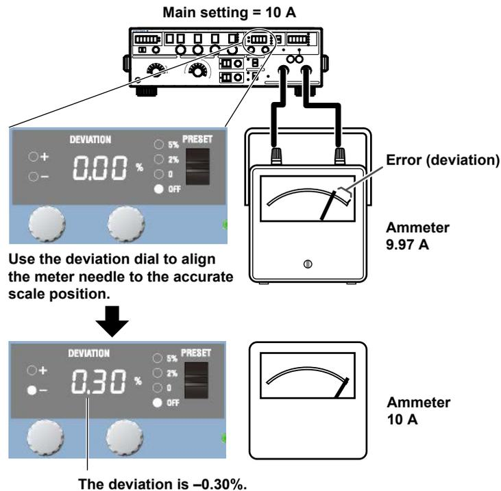
In the example above, before fine adjustment, the meter needle is pointing to 9.97 A, which is 0.30% smaller than the 10 A current output from the 2558A. The deviation polarity (the sign) of the 2558A indicates whether the target device indication is larger or smaller than the accurate position. In this example, because the meter is pointing to a value that is 0.30% smaller than the 2558A output value, the 2558A displays  $-0.30\%$ .
