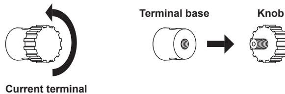
2. Insert the screw of the knob into the crimped terminal, and then tighten firmly with the terminal knob. The terminal or knob may break if you apply excessive torque.
