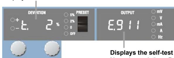
**Displays the self-test result**
