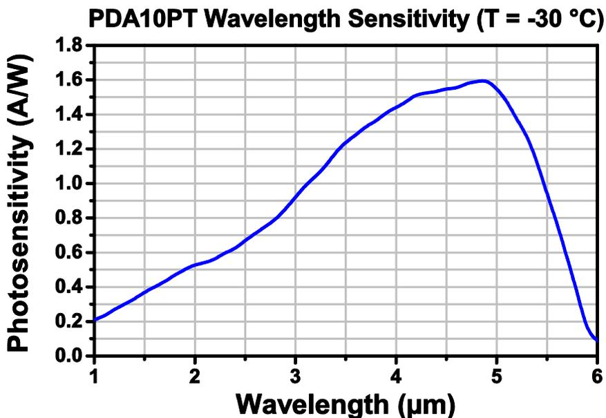
Figure 6 Wavelength Sensitivity of the Detector at 0 dB Gain Setting
