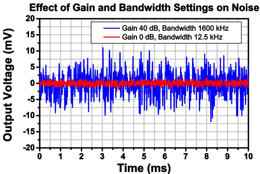
Figure 5 Noise Comparison at Min and Max Gain and Filter Settings
