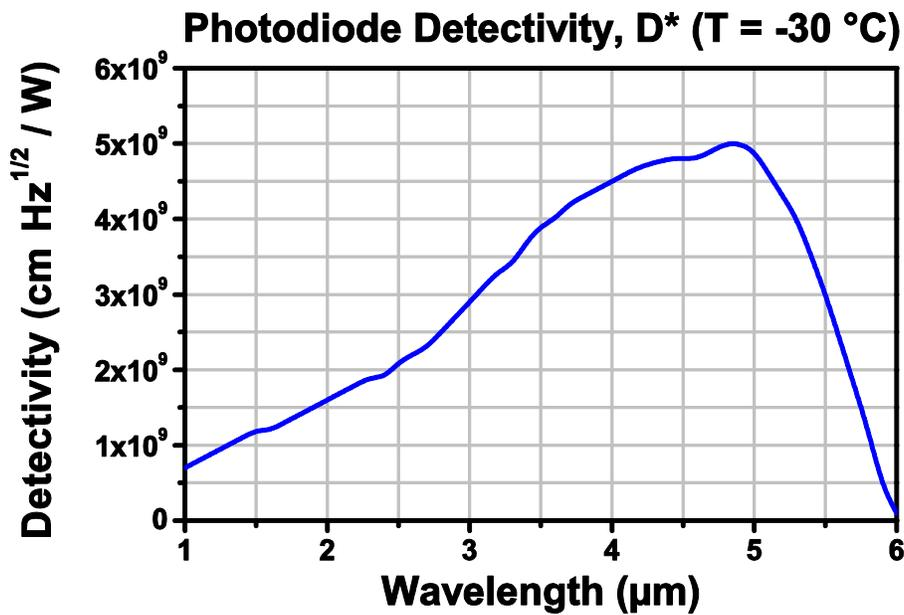
Figure 3 PDA10PT Photodiode Detectivity (D\*) at 0 dB Gain Setting
