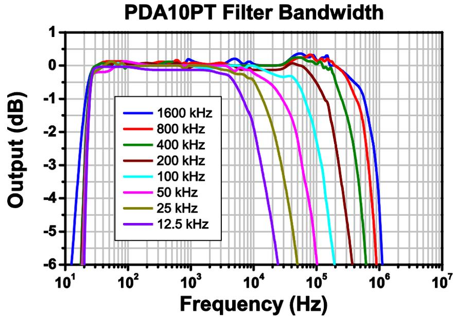
Figure 4 PDA10PT Filter Bandwidth (50 Ω Load)
