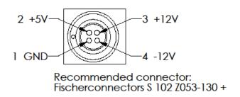
Four pole male connector on detector.
