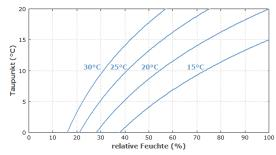
Fig. 7 : Dew point for 4 different temperatures
