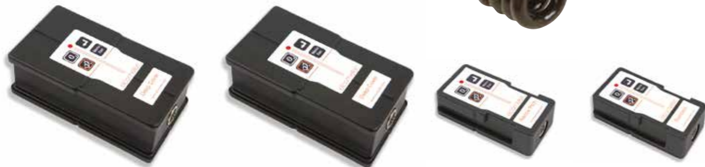
Range of fully interchangeable search heads including standard, narrow pitch, deep cover, borehole probe and half cell.
