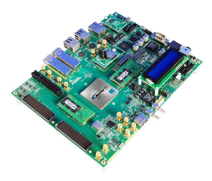
The Altera® Arria® 10 SoC Development Kit offers a quick and simple approach for developing custom ARM® processor-based SoC designs. Design productivity is one of the driving philosophies of the Arria 10 SoC architecture. The Arria 10 SoCs offers full software compatibility with previous generation SoCs, a broad ecosystem of ARM software and tools, and the enhanced FPGA and DSP hardware design flow.
