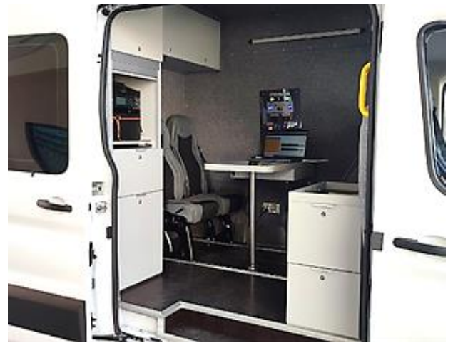
Operators' compartment consisting of MDS control panel, a laptop with RPM software, a wall-mounted alarming module
